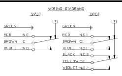
b. When making wire connections disconnect electrical power. Check for multiple circuits.
