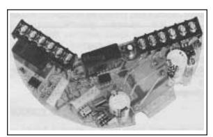
If your application requires switching in addition to local indication, our all solid state "Locked Logic" system is the most accurate available. With no moving cams, levers, etc. it does not affect the accuracy of the gauge on which it is installed. Switch accuracy is the same as the gauge accuracy.
