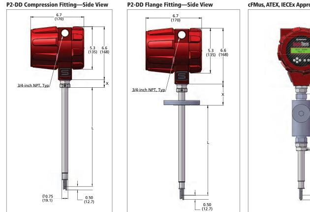
Note: All dimensions in inches with (mm) in brackets; certified drawings available upon request. All drawings have ± .25 inch (6.4 mm) tolerance.
