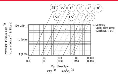
Notes: (1) For air and nitrogen at 20°C temperature and 1 atmosphere pressure (2) 1 inch of water at  $60^{\circ}F = 0.0361$  psi
