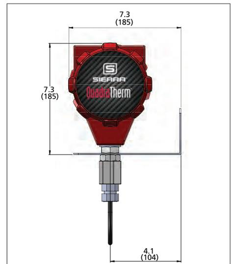
Note: All dimensions in inches with (mm) in brackets; certified drawings available upon request. All drawings have ± .25 inch (6.4 mm) tolerance.
