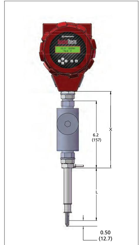
Note: All dimensions in inches with (mm) in brackets; certified drawings available upon request. All drawings have ± .25 inch (6.4 mm) tolerance.
