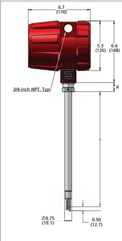
P2-DD Flange Fitting—Side View
