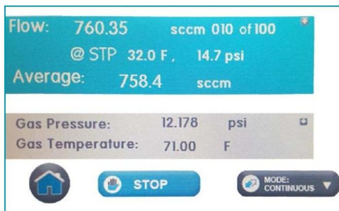
The Measure screen allows you to capture and observe instantaneous flow data. During operation, the measured flow rate, reading number, standardization information, and average readings are displayed at the top. Gas pressure and temperature inside the tube are displayed on a constant basis regardless of whether the unit is operating.
