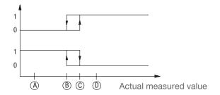
The diagram shows: Out 1 set to FSL Out 2 set to FSH 1 = contact closed
