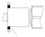
The quality of the welding with the container wall must be according to the respective regulations (e.g. gaps, transitions, surface finish).
