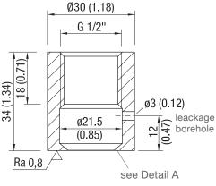
Detail A: Sealing area between CN 7120 (PEEK) and the on site process connection (metal)
