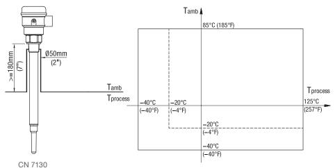
Ambient- and process temperature limited to  $-20\,^{\circ}\text{C}$  (-4 $^{\circ}\text{F}$ ) with option FFKM seal O-ring
