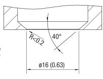
Flush welding socket: Installation
