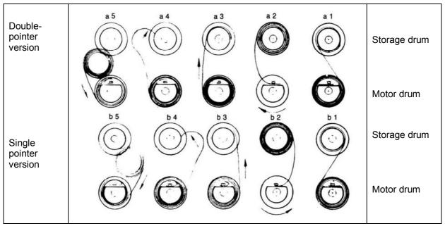
fig. 08: Instruction to wind up motor druml
