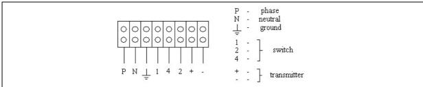
fig. 07: Terminal / Electrical connections
