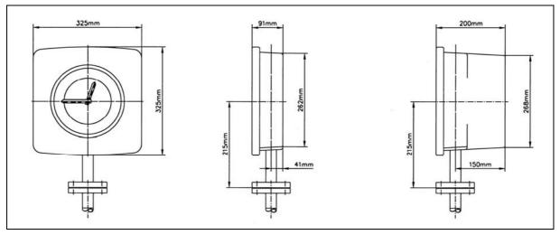
Fig. 02: Maglink-head with flat housing with wide housing
