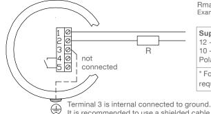
Rmax = (Vsupply -12 V)/ 20 mA Example: 24 V supply allows Rmax of 600 Ohms
