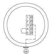
Terminal 3 is internal connected to ground. It is recommended to use a shielded cable for stable measurement.
